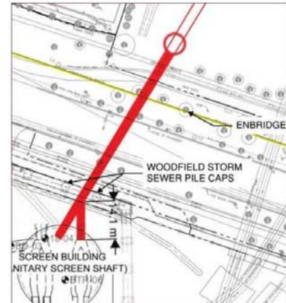
Figure 7. Alternative 3 – Launch Microtunnel from the Rugby Field at an Angle; Hand Mine or Open Cut 14 m Section Perpendicular to Screen Inlet.
